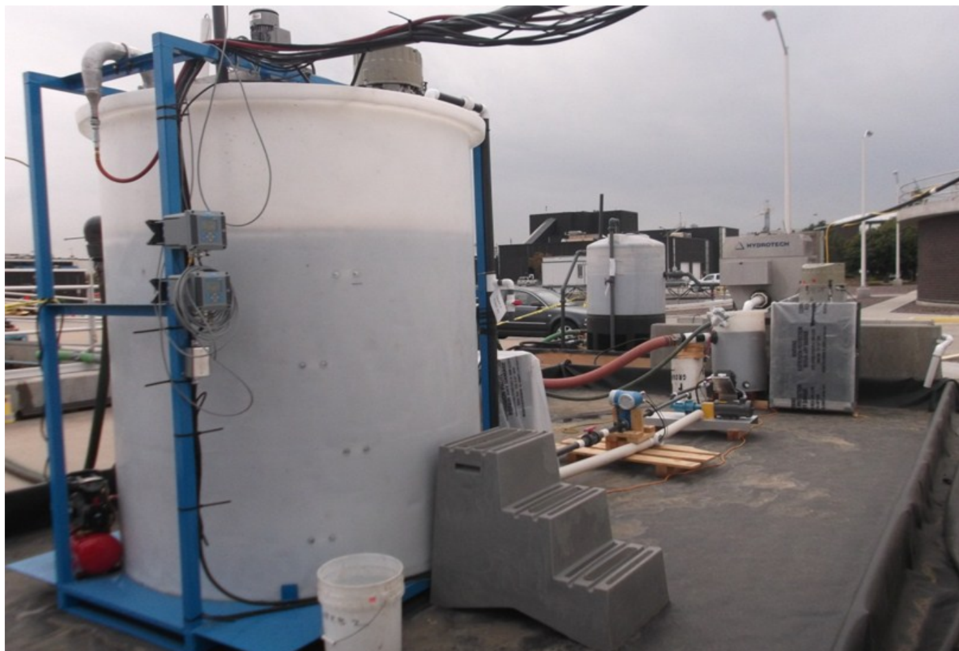
Anammox pilot study side stream biofilm reactor at Metro Wastewater
